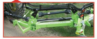
Placement of the tires are very important! The left tire tracks on top of the road. This creates a holding position to prevent side drafting. The right tire is placed directly on the hingeline of the center section and right wing, where the blades intersect. This is the best placement for a tire as the blades pick up the only wheel track and prevents almost all stripping. Competitive arms use two tires in the ditch and will tramp down more grass, causing it to strip.
