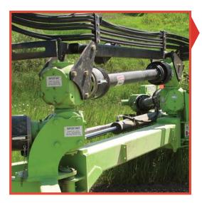
Schulte's new generation FLX-1510 sets the standard in offset mowing technology. This FLX-1510 incorporates a set of swivel gearboxes & one right angle gearbox to allow smooth transmission of power in any direction from directly behind the tractor to fully offset to the right.
